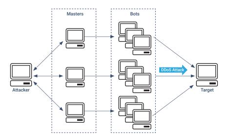
In a Distributed Denial of Service (DDoS) attack, an attacker uses multiple sources, (such as distributed groups of malware infected computers) to orchestrate an attack against a target. As illustrated in the following figure, a network of compromised hosts participates in the attack, generating a flood of packets or requests to overwhelm the target.
